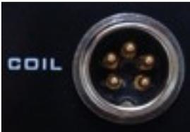
*The COIL connector serves for connection of the search coil of the metal detector to its electronic block.*
