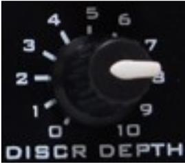
*The DISCR DEPTH potentiometer serves for adjusting the depth of discrimination (the maximum depth to which the metal detector distinguish the metals).*
