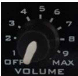
*The VOLUME potentiometer serves as the on/off the metal detector (level "OFF") and to regulate the audio volume (levels from "1" to "MAX").*
