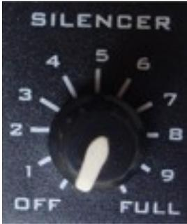
*The SILENCER potentiometer serves for setting of the degree of suppression of the background sound.*
