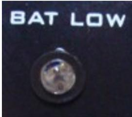
*The BAT LOW LED shows the available charge in the LiPo battery. When this LED lights up, it is a signal for low battery.*
