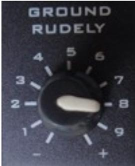
***The GROUND RUDELY potentiometer serves as a coarse (base, fast) setting of the ground balance in a manual ground balance working mode, ie for a base eliminate of the ground effect at work in a manual ground balance working mode.***
