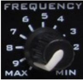
**The FREQUENCY potentiometer serves to change the operating frequency of the metal detector in range  $\pm 60\text{Hz}$ , in order to avoid external interferences such as: interference from other close working metal detector with the same or similar operating frequency; and powerful industrial interferences.**
