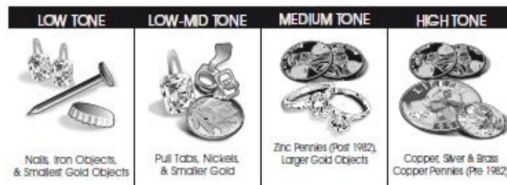
Audio Target Identification (ATI) clasifies metals into four categories.
