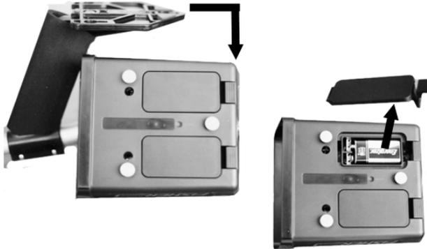
*If either or both of the batteries are installed incorrectly, the Gold Strike will simply not turn on. The detector will not be damaged.*
