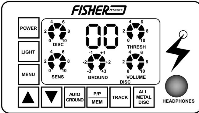
1. The POWER button turns the unit ON and OFF. One of the first things you will notice when you turn on your Gold Strike is the battery level display. Fresh batteries will show 9 volts; when the battery level is down to 6 volts, you have a little more than an hour of battery life left. The detector will not turn on if the search coil is not properly connected. This can prove to be a timesaving safeguard.
