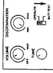
If the pointer on the view meter is between 3 and 6 (green area), the batteries have enough power to operate the detector. If the pointer is not in the green area, replace the batteries.
