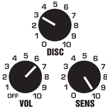
**HEADHUNTER** DIVER & WADER models have three controls for the micro-encapsulated circuitry located in one sealed earcup of the headphones. Batteries are found in the other earcup and are user accessible.
