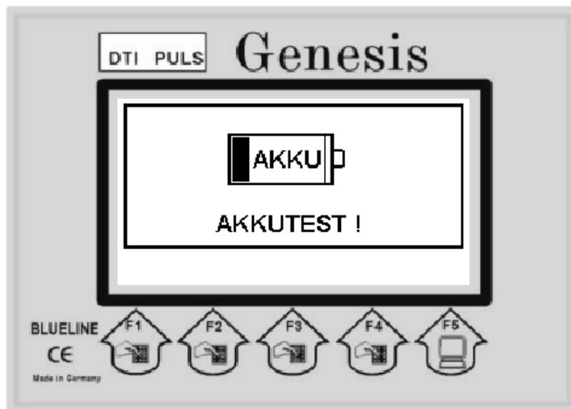
A beep will be produced. The condition of the rechargeable batteries will be checked. If the rechargeable battery is not ready for operation a message will be displayed. You have to switch off the detector for charging batteries.
