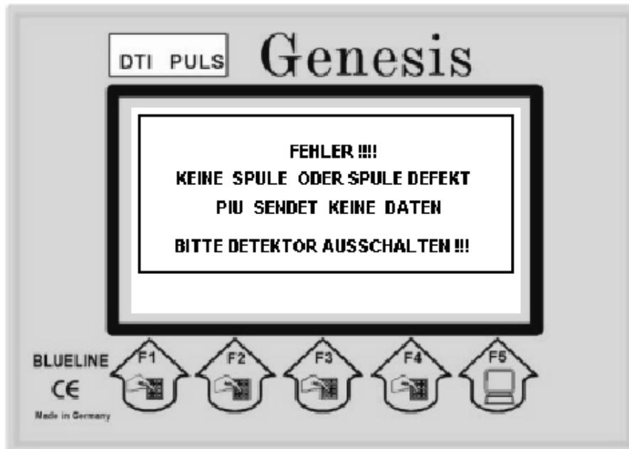
When you choose a start with coil without having connected a coil this message will be displayed. The system switches to the demonstration mode.
