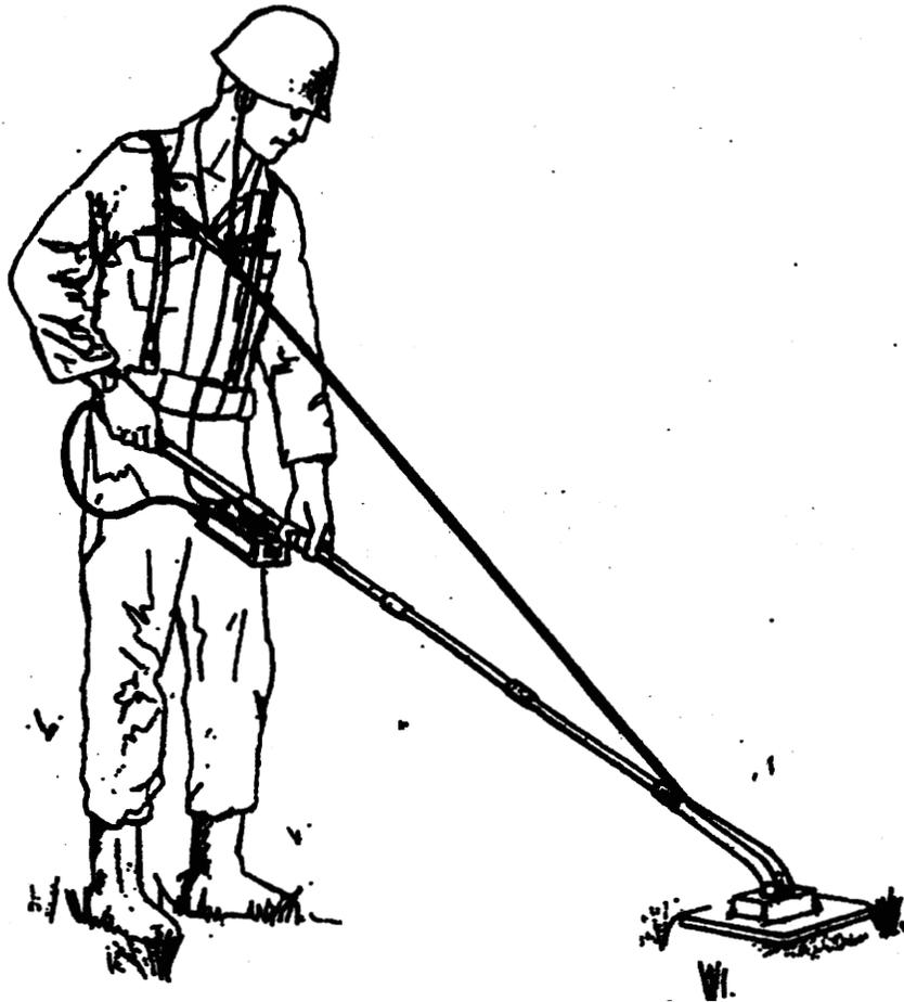
**Figure 2-3. Mine Detector Operation in Standing Position**
